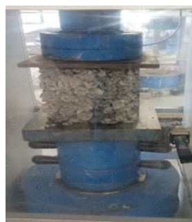
Figure 3. Compressive strength testing.
