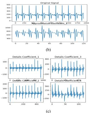
FIGURE 4. (a) Results of the respondent's signal on the ECG paper. (b) The original signal on the module and the results of the approximation coefficient level 4. (c) The results of the details coefficient level 1 to 4.
