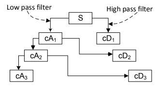
FIGURE 3. Details Coefficient and Aproximation Coefficient from Discrete Wavelet Transform Decomposition
