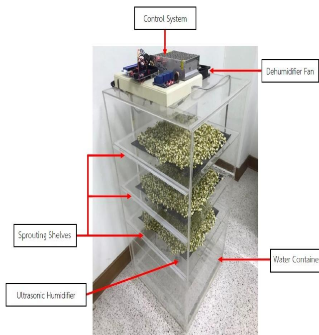
Fig. 3 The components of the temperature and relative humidity controller (in the isometric view)
