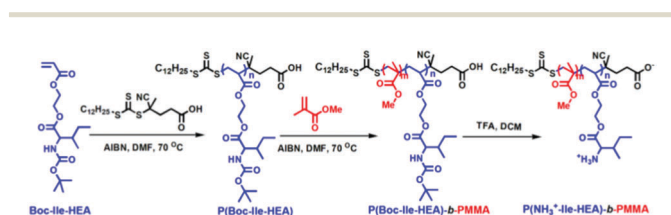
Fig. 1 A schematic representation of RAFT mediated block co-polymerization of Boc-Ileu-HEA and MMA monomers, followed by deprotection of the Boc group to enable proton exchange between the hydronium and labile amine groups.
