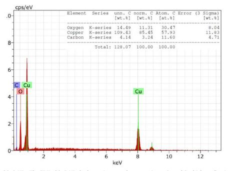
Fig. 4: EDX spectrum of CuO-NPs. The EDX of CuO-NPs had prominent peaks respective to Cu and O which confirming synthesis CuO-NPs. The peak for carbon was due to the carbon tape used for mounting the sample on aluminum stub before analysis
