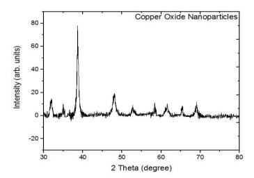
Fig. 2: XRD spectrum of CuO-NPs. The clear and strong peaks corresponding to 20 values of 32.10,35.40, 38.20, 4840, 53.50, 58.10, 61.20, 65.50, 67.30 for the respectively marked indices of (110),(002), (111), (202), (020), (202), (113), (022), (113) respectively and indicating the formation of CuO NPs
