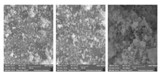
Fig. 3: FE-SEM images of CuO-NPs. (a) 500 nm (b) 200 nm) the results revealed the formation of slightly agglomerated spherical NPs
