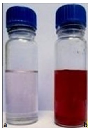
a. Aqueous extract of algal powder before the formation of silver nanoparticles b. Silver nanoparticle formation in aqueous crude extract after the addition of silver nitrate
